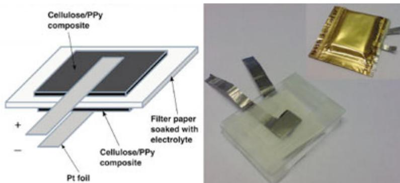
*The Cladophora cellulose-polypyrrole conductive paper composite. Left: schematic image, and right: photograph of the composite paper battery cell before and after sealing it into a polymer coated aluminum pouch. (Reprinted with permission from American Chemical Society)*
